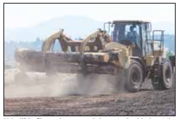
Idaho White Pine sawlogs are on their way to the debarker at the sawmill, courtesy of Terry Thomas' CAT 966.
