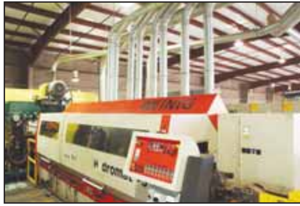
After rebuilding due to a fire that almost completely destroyed the operation, this Weinig moulder facility was installed.
