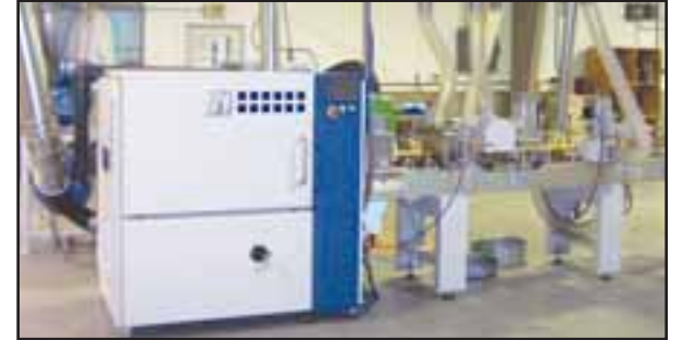
Durgin & Crowell's Enhanced Paneling and Flooring travels through an 8-head profile sander before being processed in the Delle Vedove vacuum coated UV curable paint machine.
