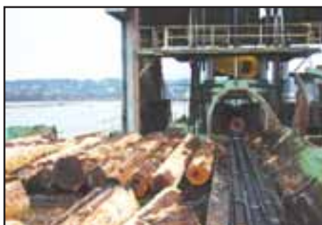
This is a photo of a debarker discharger at the Bridgeview Mill in Surrey, B.C.
