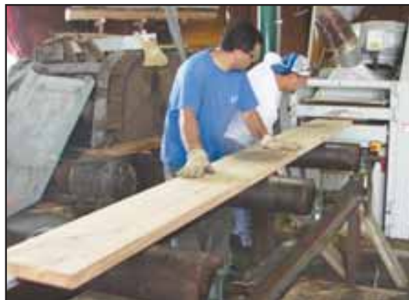
Richardson employees are shown surfacing all four sides (S4S) of a 2x12 Douglas Fir timber.
