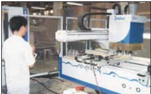
A Pacific Traders worker shapes wood parts using a CNC router.
