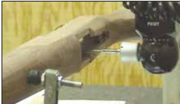
A Walnut rifle stock is measured by the Computerized Measuring Machine (CMM) during the production process.
