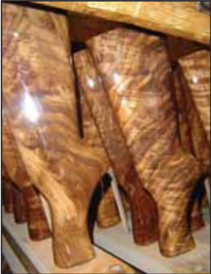
Finished Ultra Walnut shotgun stocks are lined up for the checkering machine.
