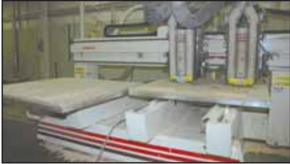
One of Automated Routing Inc.'s woodworking machines is working on moulding that goes around an examination table.
