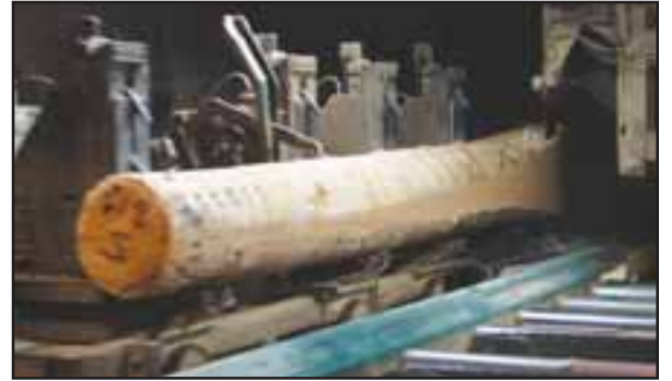
Eastern White Pine sawlog is sawn by a double cut bandmill.
