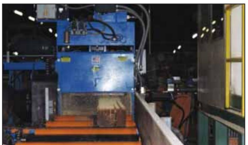
Bradford's ASM refurbished 8-inch gang saw outfeed is pictured here.
