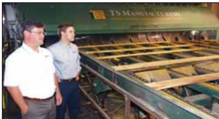
Adam Moran and Wesley Boles monitor kiln-dried lumber being trimmed after kiln-drying and inspection.
