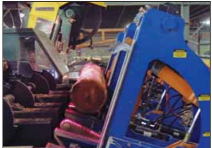
The company's ASM carriage and Filer & Stowell 7-foot bandsaw.
