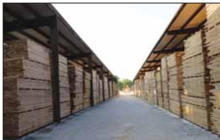
Oak is pictured under air-drying sheds prior to being moved to the kiln-drying operation.
