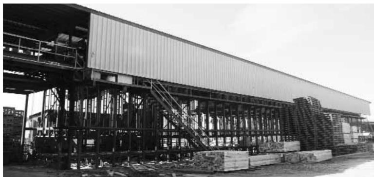
This is a picture of Independence Lumber, Inc.'s 60 bay bin sorter located at their band mill operation in Independence, VA. They also have a planer at this operation.
