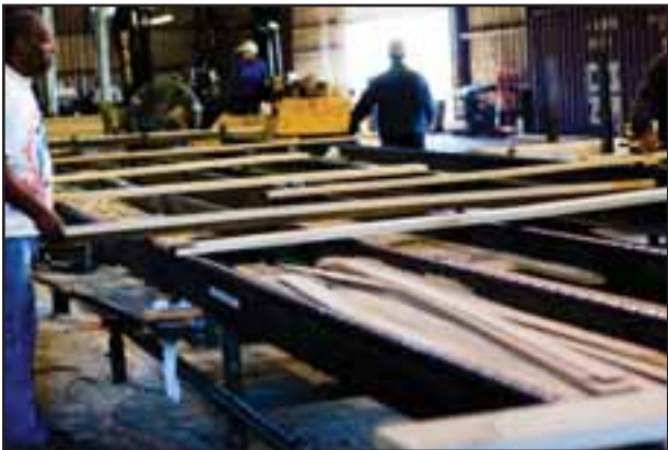
Ripped or fixed-width strips coming off the chain are pictured here.
