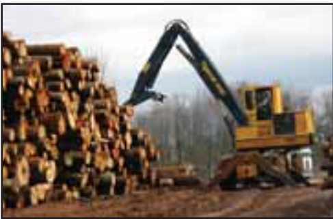
Thompson Appalachian Hardwoods procures logs from a 200-mile radius. The company stores logs on a wet deck with a self-propelled Tigercat 250D and A16 carrier.
