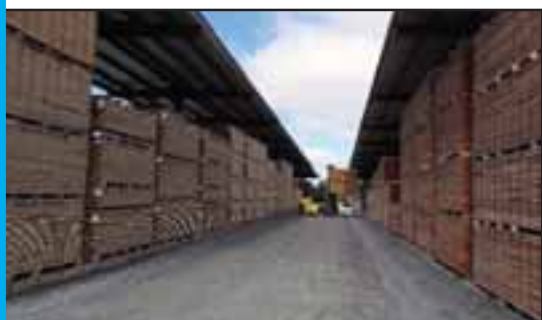
Covered air drying facilities and concentration yard in W. Springfield, N.H.
