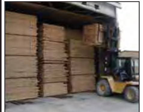
Silver Leaf Soft Maple is being loaded into a kiln. Missouri-Pacific also carries Red and White Oak, Ash and aromatic Cedar.
