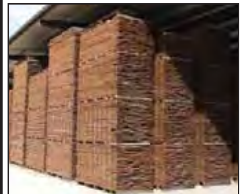
With over 1.5 million feet of covered air dry storage, Missouri-Pacific dries its thicker stock Walnut and Oak in these buildings.
