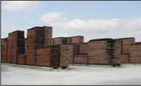
Concrete foundations in the air-dry yard, and proper stick placement, ensures flat lumber for Missouri Pacific Lumber Company's customers.
