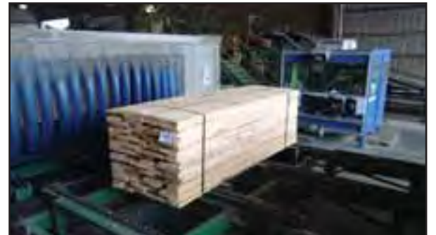
A bundle of Red Oak lumber is tallied on Hermitage's state-of-the-art picture tally and weighing scales.
