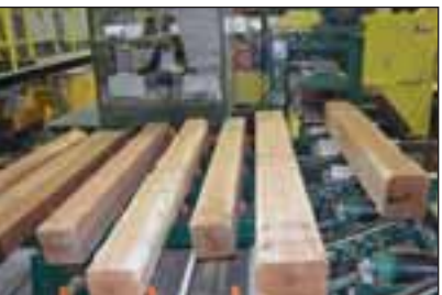
Wheeland Lumber recently installed a 62-inch McDonough horizontal resaw with McDonough MAXX In-feed and Tipple Outfeed system.
