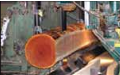
Quality lumber begins with Wheeland's fully computerized double-cut band headrig equipped with USNR 3-D scanning and linear positioning.
