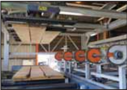
A Joulin vacuum lift feeds 5/4 12-inch and wider Red Oak into a Raimann KR450 4 moving blade optimizing rip saw.
