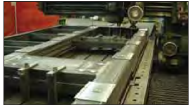
A new Corley carriage frame in the machining stage of production.
