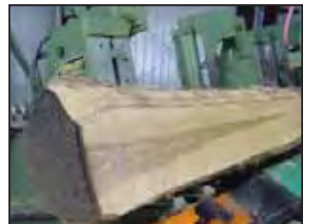
A log is shown processing through a Corley tilt carriage.
