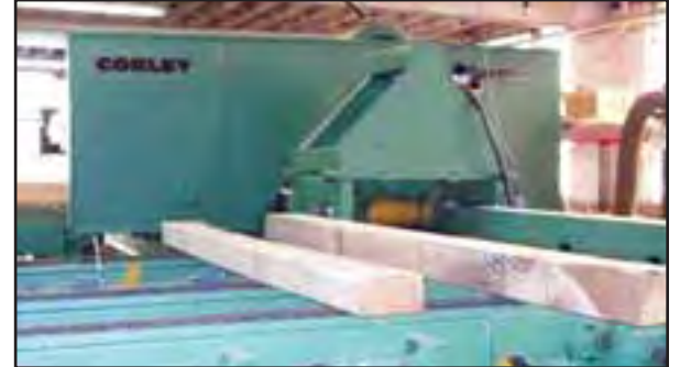
Corley's horizontal resaw shown here.
