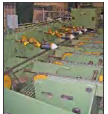
Corley recently replaced the optimizing edger system at Begley Lumber, located in London, Ky., with a new four-saw edger as well as a new Lewis optimization and scanning system.
