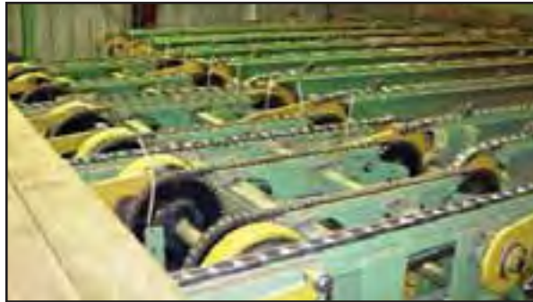
Corley board feeder in operation.
