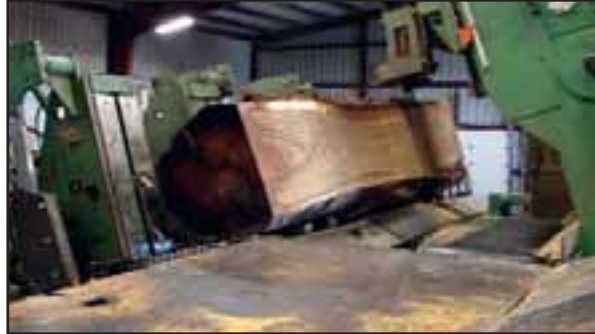
Walnut being processed on the 7-foot 17-degree slant Corley headrig.
