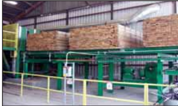
One of the Collins Cos. Tilt hoists with stickered kiln-dried lumber.
