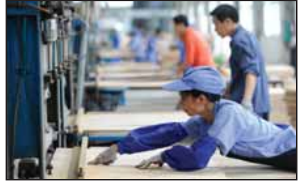
A Shelter Forest production technician operates a veneer scarf jointing workstation.
