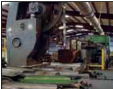
A 7-foot vertical resaw further processing a cant for grade lumber.
