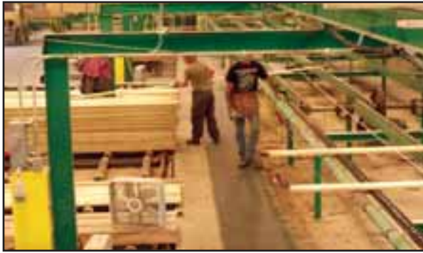
The Collins Companies Richwood, Virginia, "MegaMill" sorting chain and stacker by-passer.
