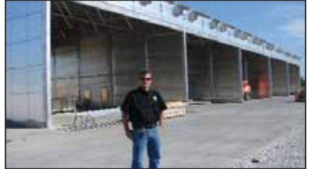
Stan Smith standing in front of Missouri Walnut's SII dry-kilns. The company has 1.53 million feet of dry-kiln capacity per charge.
