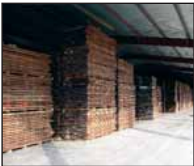
5/4 through 10/4 lumber being air-dried under Missouri Walnut's 550'x60' building.
