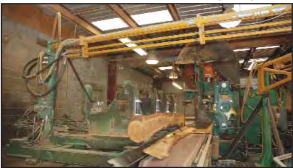
This is a view of Neff's computer operated linear positioner Corley carriage and McDonough six-foot band saw.
