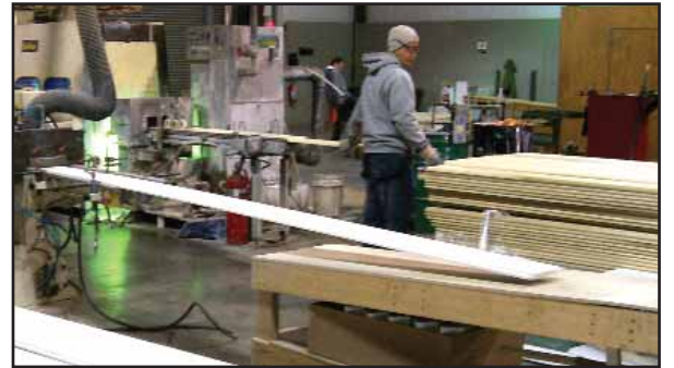
The Delle Vedove catalytic UV primer and profile sander can process up to 20,000 lineal feet per day.
