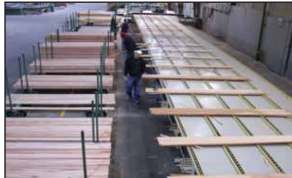
The Weing Raimann rip saw can be programmed to handle up to 10 width sorts.
