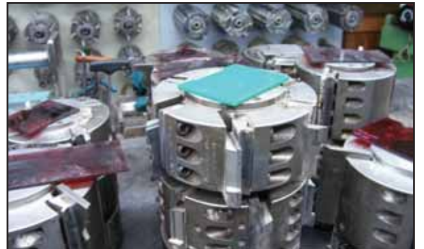
Molder heads are prepared to run thousands of custom profiles on 8 Weing molders.
