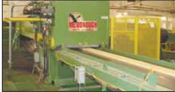
Some of the operation's major pieces of equipment are this state-of-the-art edger, manufactured by McDonough Manufacturing. According to President and Chief Executive Officer Mel Yoder, the firm has seen sizable yield increases since the installation. "This edger is a wiggle box edger with 3 movable blades. The USNR optimizer scanner gives us the maximum width board as well as a two-board solution if possible, which increases yield."
