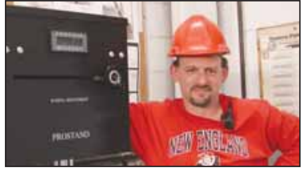
Mike Halle, Bethel planer mill manager standing by the Pro Stand radial adjustment machine, which ensures the new moulder's knife stock is 100 percent accurate.
