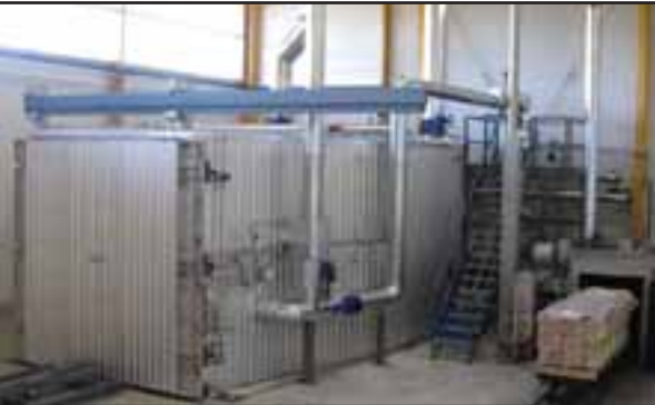
Jartek's 10,000 board foot capacity Thermal Modification Chamber with a small research chamber.
