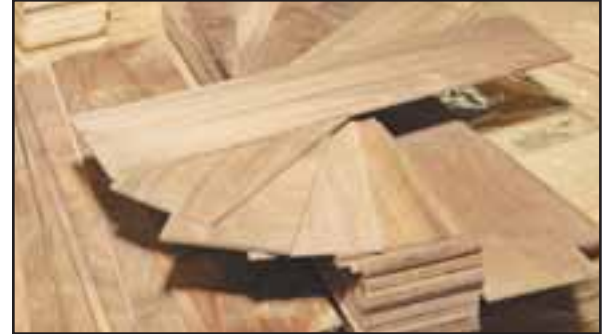
American Walnut is another species preferred at Tanjung Kreasi. Pictured are samples of lumber blanks manufactured by the firm.
