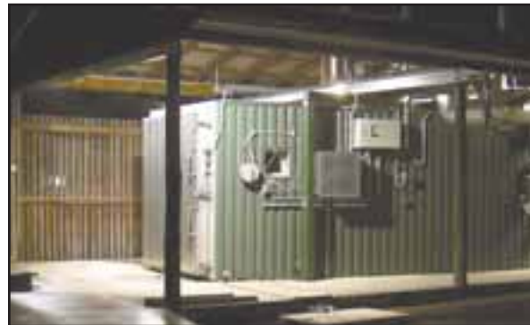
Jartek's 3,000 board foot capacity Thermal Modification Chamber.
