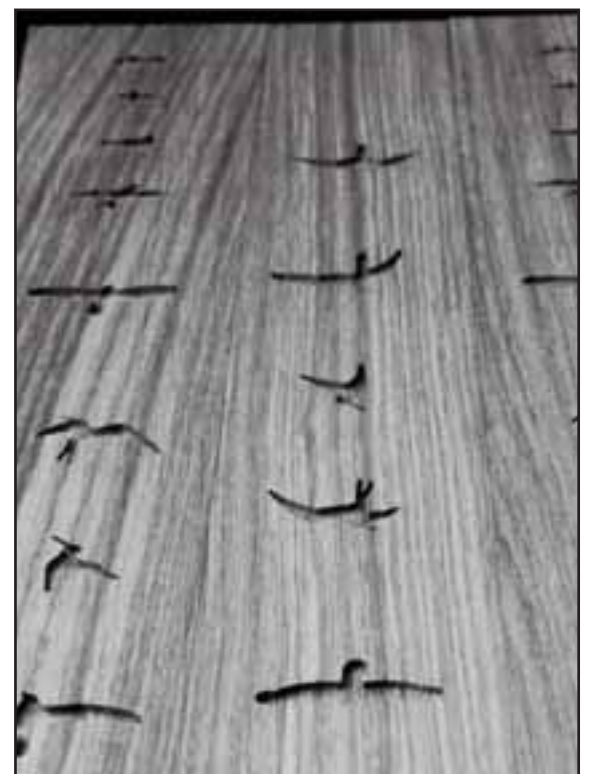
Birds are carved into Rosewood on these guitar fingerboards. PRS makes 60 guitars per day, mostly handmade.
