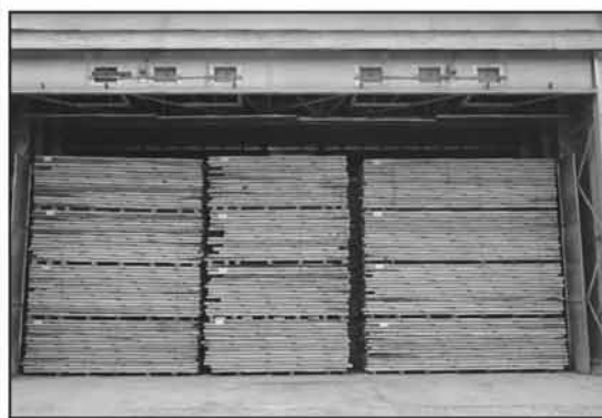
This is a view of some of Gilco International Lumber, LLC's 8/4 Poplar being kiln dried.
