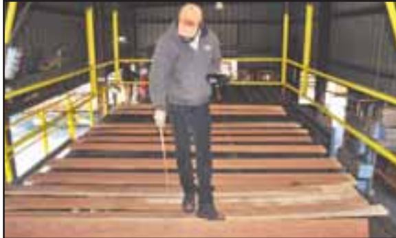
Henry Ledford grades lumber at Oaks Unlimited's green inspection and stacking chain.
