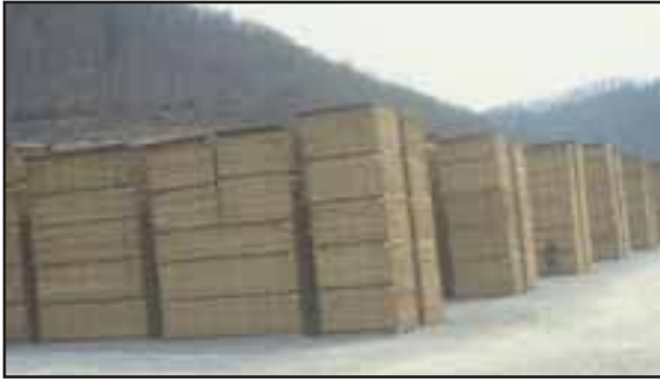
Gilco International Lumber LLC's hardwood concentration lumberyard in Roderfield, W. Va. is situated on 20 acres with a one million board foot capacity pre-dryer, 16 Irvington-Moore dry kilns, air-drying sheds and yard with four million board feet of open air-drying capacity.
