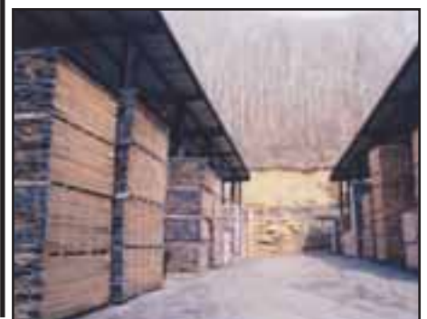
Two air-drying sheds are photographed here at Gilco International's hardwood concentration yard in Roderfield, W. Va.
