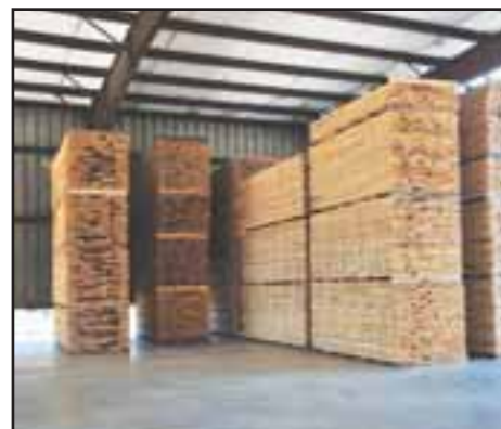
Green lumber under the company's covered air-drying facility.
