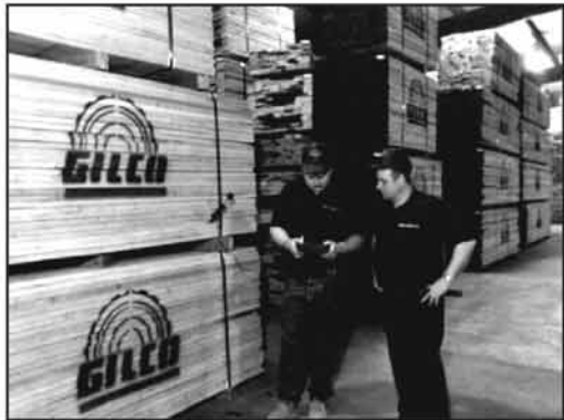
David Hagerman and James Ray checking moisture content in lumber at Gilco's Roderfield, W. Va. facility.
