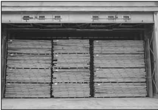
A view of 8/4 Poplar being kiln dried at Gilco's new hardwood concentration yard in Marion, N.C. This new yard will produce an additional 15,000,000 board feet of kiln dried lumber annually.
