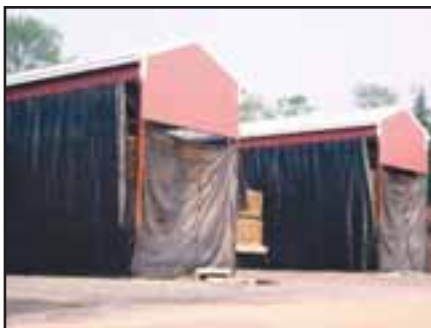
These T-sheds help keep lumber that is being air-dried protected from the elements.
