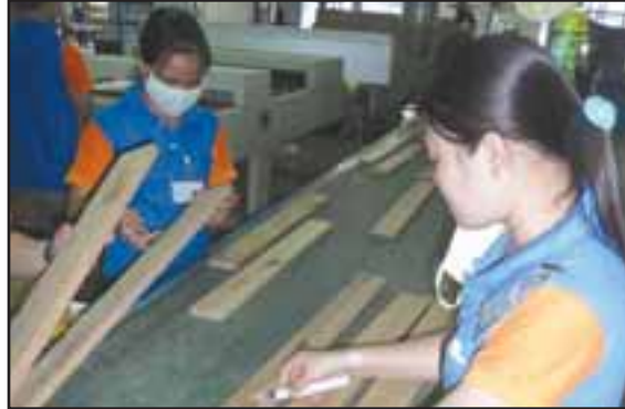
Production management is based upon a product flow, rather than a batch system, and minimizes "Work In Progress" with components drawn, as needed, from a central material pre-prepared stock.
