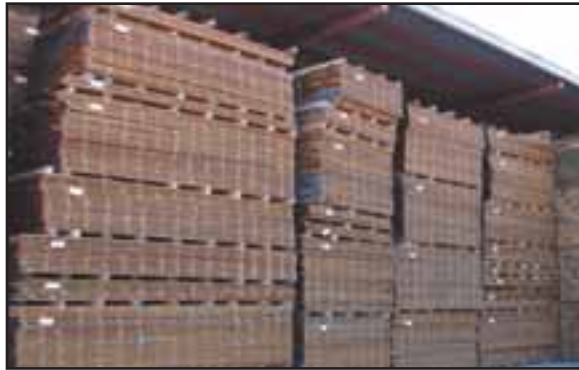
lpe is air-dried under a cover at Baillie Lumber Co., headquartered in Hamburg, N.Y.
