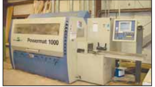
The Weinig Powermat 1000, six spindle planer/moulder, with 12,000-RPM spindles, is used to produce the company's mouldings.
