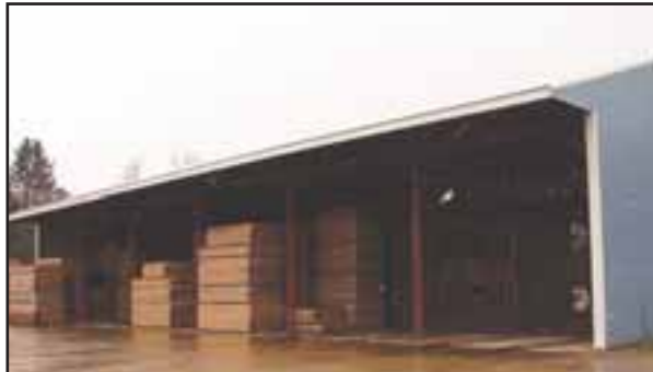
Bingaman & Son has a 240,000-board-foot fan drying shed to maintain excellent color in whitewoods during the summer months.
