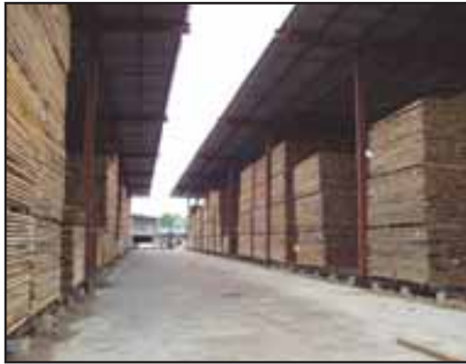
This photo shows hardwoods air-drying in two of the company's T-sheds. Hardwoods of America has 6.5 million board feet of T-shed capacity.
