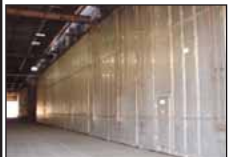
This photo shows three of Hardwoods of America's 12 computer-controlled dry kilns, each with a capacity of 100,000 board feet.
