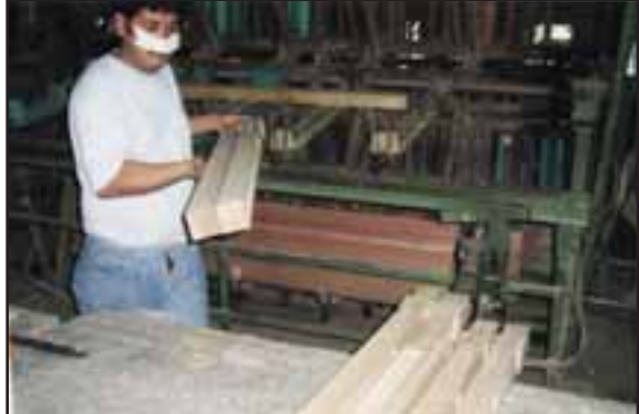
Lamination involves putting sawn lumber pieces together for the production of larger furniture items.
