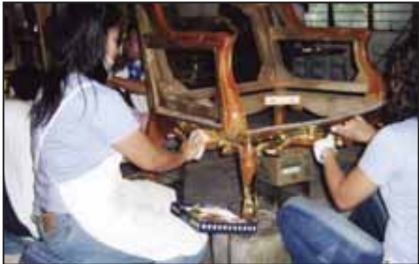
Gilding, which is used at JB Woodcraft’s facility, involves the application of a layer of gold over furniture parts.
