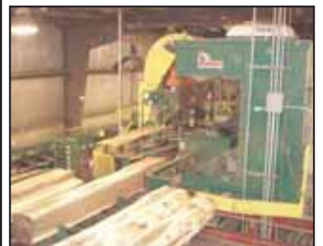
This shows a Black Walnut cant feeding into a McDonough linebar resaw.
