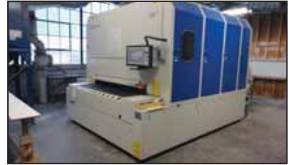
Additional equipment operated by the company includes a Heesman brand veneer sander with a maximum width of 64 inches.
