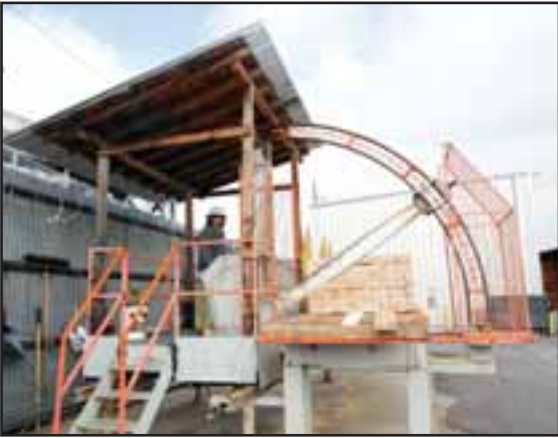
A Transcut II station manufactured by Holtec, Plant City, FL, cuts units of lumber for crating material.
