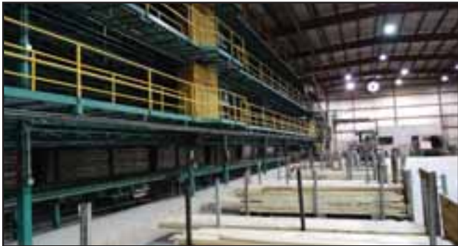
Pictured is the tray sorter at Devil's Tower Forest Products, Neiman Enterprises' first location.
