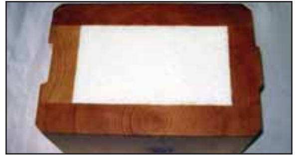
The core of the Cedar Yurt log is a solid piece of EPS foam encased by solid wood. This doubles the R-Factor of a typical solid log wall, and is engineered and designed to be half the weight of a typical full log.
