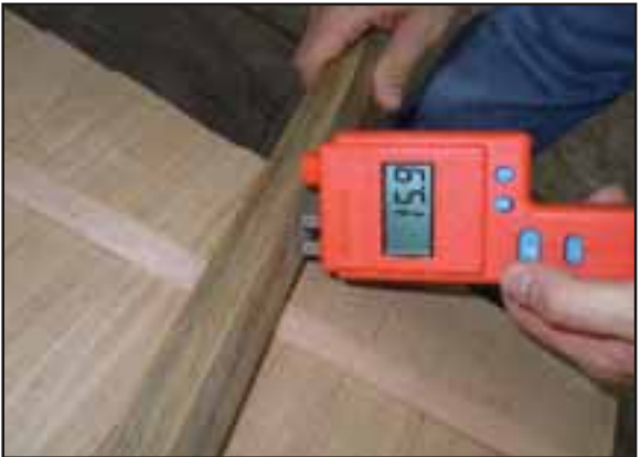
Moisture content inspection is performed on all materials at Downes & Reader Hardwood Company, located in Stoughton, MA.
