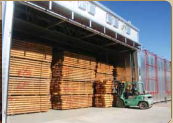
(ABOVE) Golden Eagle's 100,000-board-foot capacity SII kiln is used to dry much of the raw product onsite to 15-19 percent, and Pendu equipment carries logs through every step of the production process from shaping to planing.
