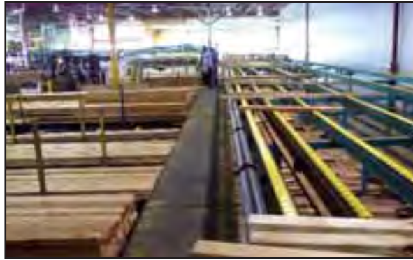
Plastic chains throughout to reduce iron stain
