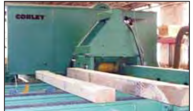
Corley's horizontal resaw is shown here.
