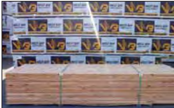
Finished Western Red Cedar products are packaged with bottom protection and 100% plastic banding to reduce iron stain.
