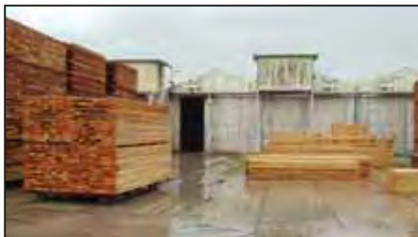
The company currently operates 10 dry kilns, which hold 250,000 board feet each.
