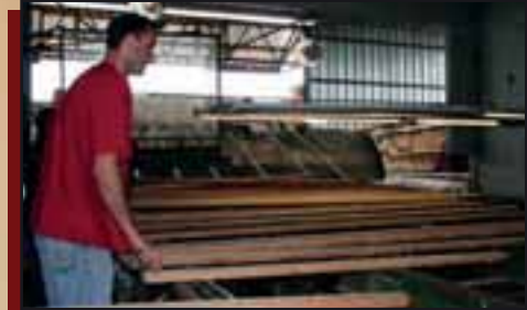
Dry Chain – We are one of the few companies that re-grades all industrial clears after drying, ensuring we don't pass along defects resulting from the drying process.
