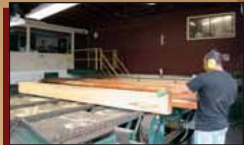
Edger – Our Shurman edger has 12 movable saws allowing us to cut flitches up to 6 inches thick into a variety of products and grades in one pass.
