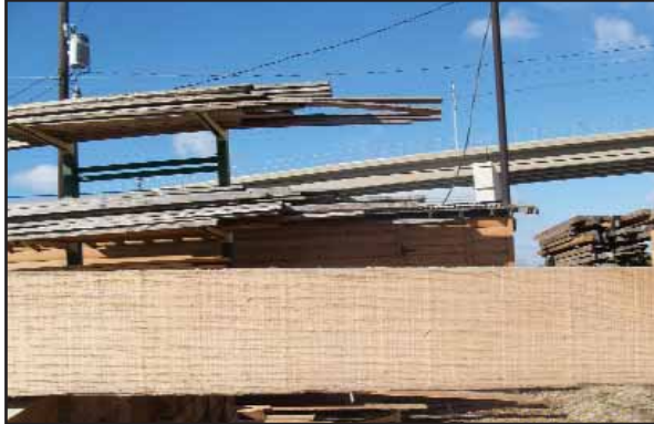
After the Tru-Ruf machine's four saw blades process the timber, the appearance is a fresh cut timber.
