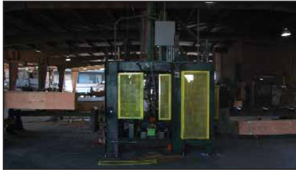
Custom built Tru-Ruf equipment provides a fresh cut appearance to the timber once it is processed.
