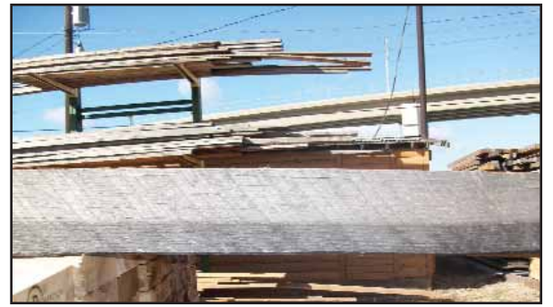
Mineral stains, banding marks and graying of timbers often come with the territory of carrying inventory. A timber is shown here before running through the Tru-Ruf machine.
