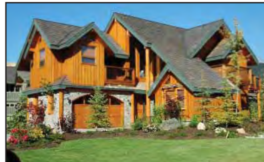
Wood siding is a board-type weatherproof product applied to a building as a final surfacing for exterior walls. Western Red Cedar siding is produced in various dimensions and different profiles (shapes) including bevel, board and batten, tongue and groove, and channel.
