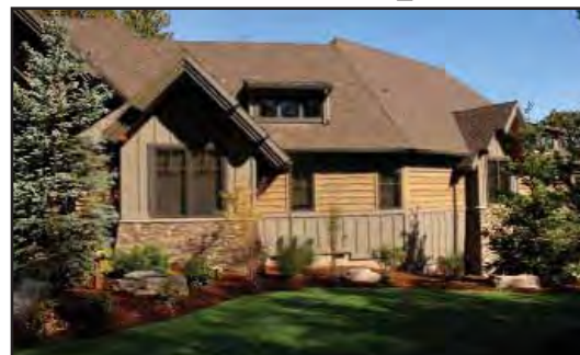
Wood siding is a board-type weatherproof product applied to a building as a final surfacing for exterior walls. Western Red Cedar siding is produced in various dimensions and different profiles (shapes) including bevel, board and batten, tongue and groove, and channel.
