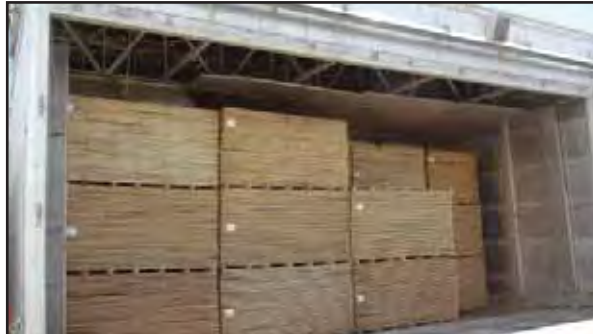
Sil Dry Kilns, loaded with Pacific Albus lumber.
