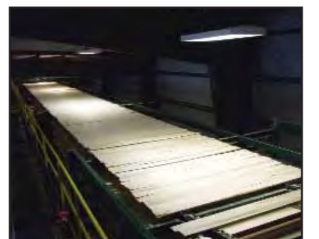
Tray sorter—gentle on the lumber after surfacing and during packaging.
