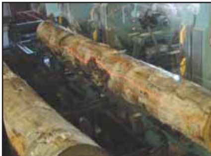
A new HMC circular saw carriage with Jacobson electric drive, have contributed to sawing accuracy and consistency.
