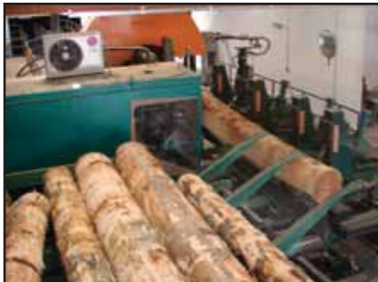
DiPrizio's new Sanborn 7-foot double-cut band saw with a Cleereman carriage and electric drive are shown here.
