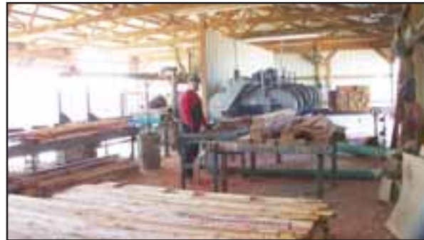
Northern Kentucky Cedar uses a six-head Wood-Mizer resaw to produce specific dimensional lumber for customer orders.
