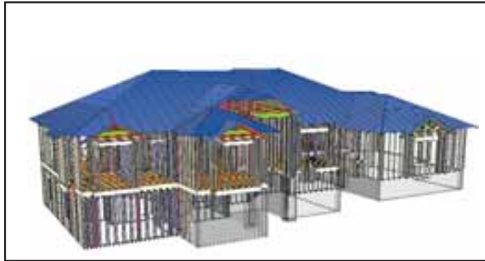
Software offered by iLevel is specifically designed for dealers to work with their builders to optimize the frame of a house. This is an image from the companies Javelin software of a 3-D model that allows movement of the house up to 360 degrees. This software will update the lengths and connections of all members resulting from any change and revise the material list.
