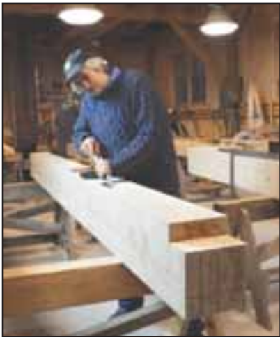
A Sweet Timber craftsman cleans out a mortise pocket with a 2-inch framing chisel.
