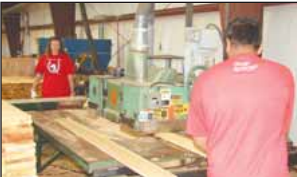
This is a photograph of 1x6 Western Red Cedar being ripped to 1x4 with an automatic rip saw.
