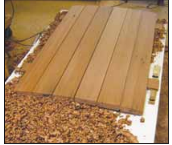
This photo, provided by Dialogue Design-Build, is of a set of solid curved doors milled from 3x8's provided by The Lumber Baron. The doors will be installed at an amphitheatre.
