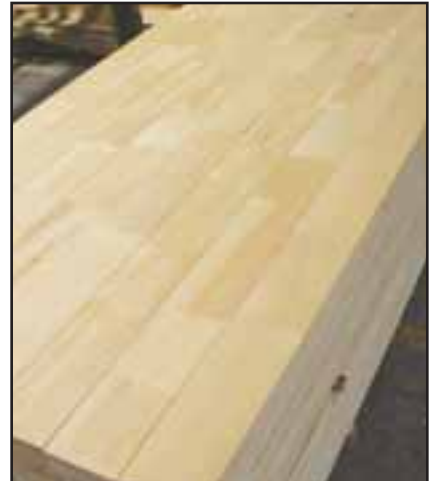
Finger joint blanks are stacked on custom milled stickers to hold them perfectly straight during the overnight drying process.
