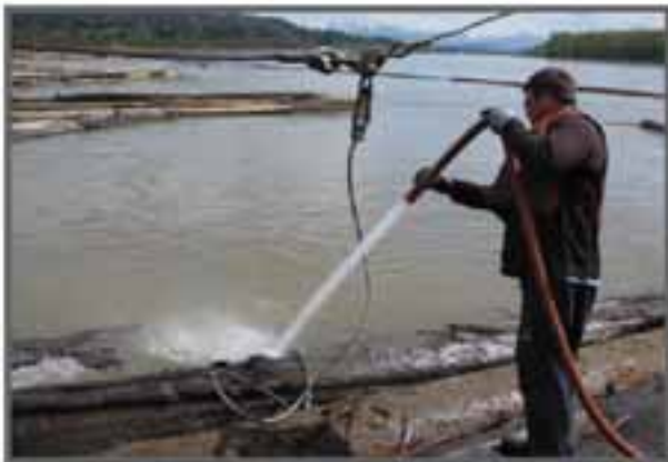
Logs are washed to remove rocks, mud and other debris that effect the saws that are clean, sharp, and precise.
