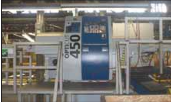
A Weining 450 Opti-cut, known as "the fastest saw in the world," carries out the cutting solution provided by the Luxscan scanner.
