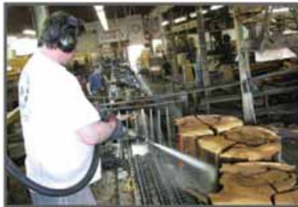
On the deck, the blocks are washed to ensure clean sawn faces.
