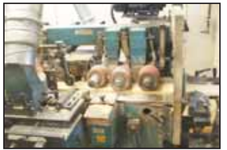
Mill Services uses one of two Watkins moulders to create a smooth, high quality finish.
