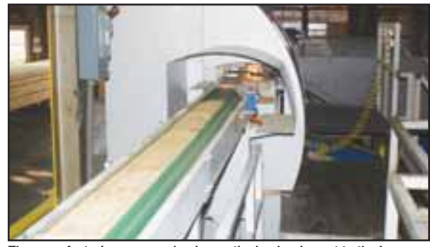
The manufacturing process begins as the lumber is sent to the Luxscan scanner to identify defects. Six separate cameras scan each board and record the information.
