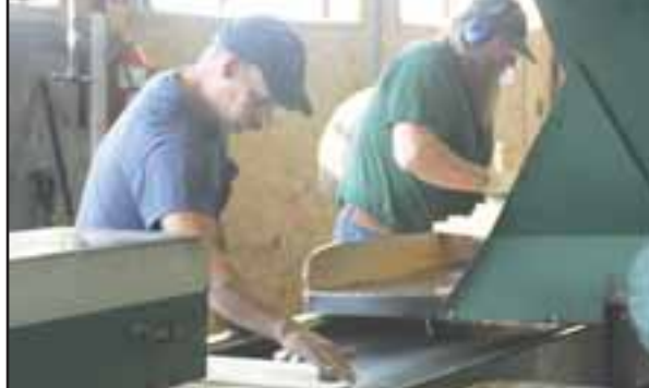
Blocks are carefully inspected at multiple points before they are fed into the CRP 2000 finger jointer.
