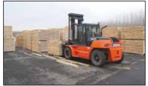
Collins Pacific Albus lumber is first well air-dried in the central Oregon sunny, dry and breezy climate before heading to the kilns.
