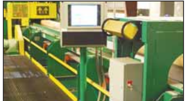
A cant is sawn by a TMT curve gang saw, following any curvature in the cant. The TMT provides higher recoveries, straighter lumber and less slope-of-grain in the lumber, compared to conventional gang saws.
