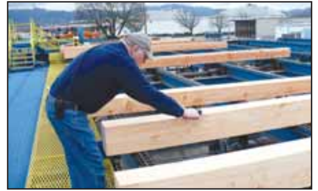
Jim Hardeman measures timbers with calipers in quality control.
