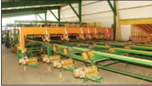
This photo shows the infeed to Wynn timer's three slowdown grading stations.
