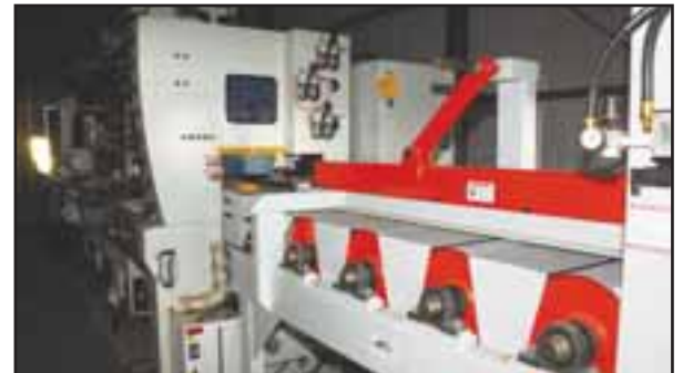
This is a photo of the infeed to the Super Thundermac moulder.
