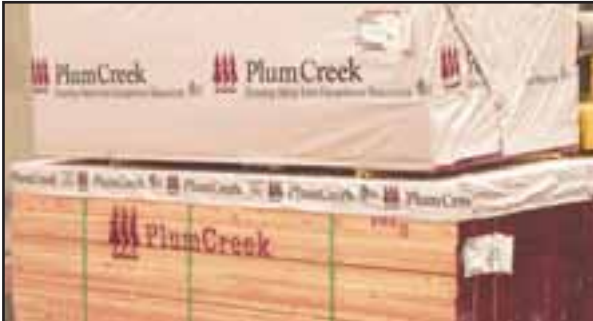
Some solid Fir-Larch studs are shown stacked in the warehouse.
