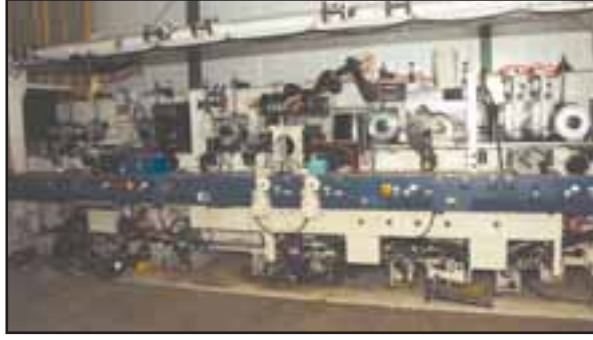
Wynn timer recently installed a LMC 2008 Super Thundermac planer/moulder, which is 9-feet wide, 24-feet long and weighs over 80,000 pounds.
