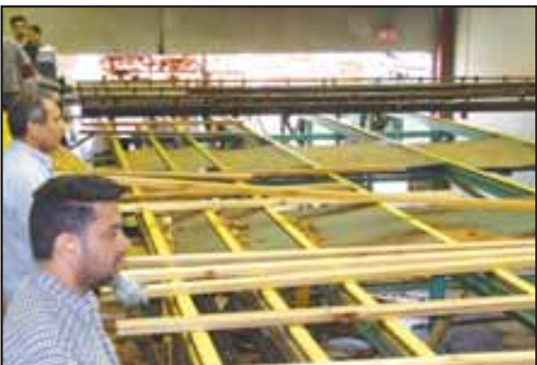
The company’s indoor green chain has plastic caps to prevent iron stain.
