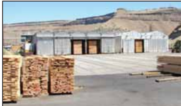
The facility, which nests along the banks of the Deschutes River near the Cascade Mountains, includes five Nardi and two Wellons dry kilns, with a capacity of 700,000 board feet per charge.
