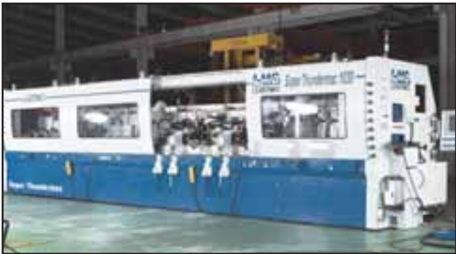
A Super Thundermac, the first planer/moulder of this size to deliver into North America, will be at the core of Wynndel’s new finish line.
