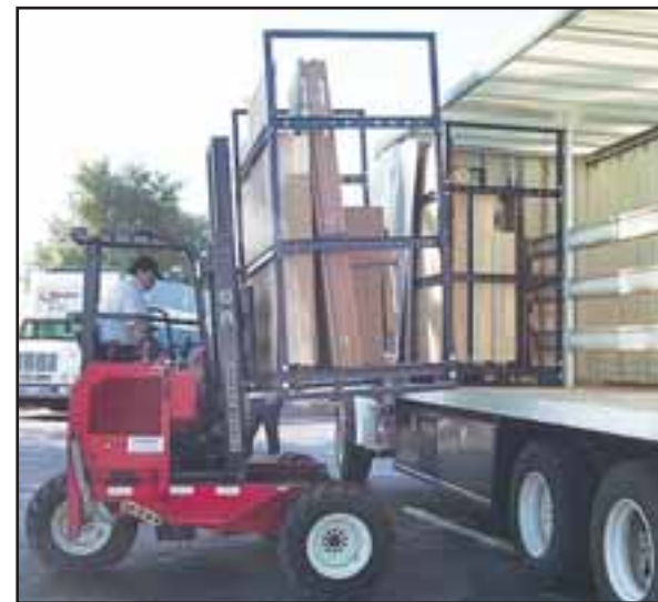
A forklift loads a door and window rack for delivery.
