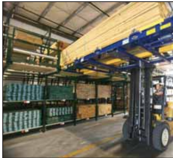
A Power Deck loads a bundle of lumber on the third level of the Power Bin system.
