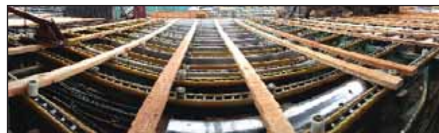
West Bay's production facility has plastic green chain to reduce iron stain.
