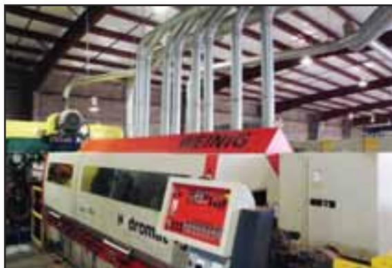
An eight-head Weinig moulder is utilized in the product manufacturing process at Pacific Western Wood Works.
