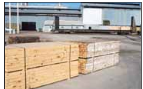
Southern Yellow Pine, Green 4x4, Mycostat™ treated vs. non-treated, 45 days old on yard in Arkansas.
