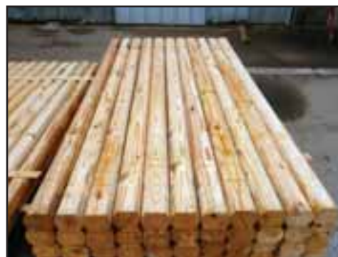
Mycostat™ treated Green Southern Yellow Pine, peeler cores, 2 months old.
