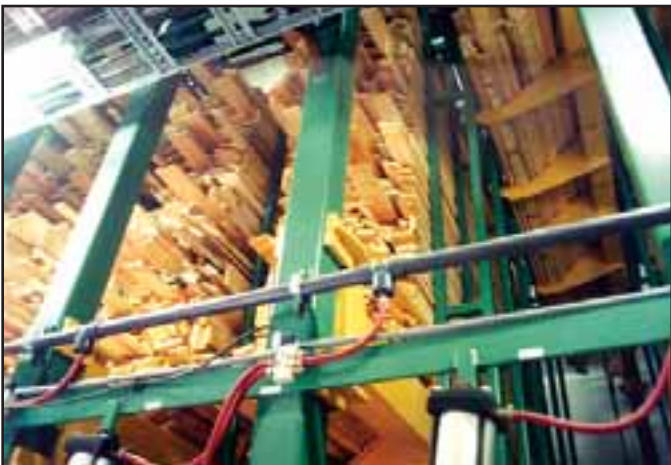
TS Sorters are installed in softwood mills working at over 150+ lpm.
