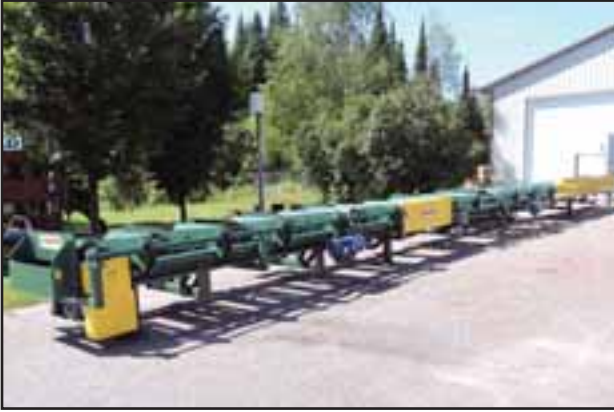
This is Cleereman’s High Speed 4-Way Sort Table.
