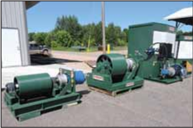
The equipment is as follows, from left to right: 100 HP Hydrostatic Cable Drive, 150 HP Hydrostatic Cable Drive, 50 HP HPU for Cleereman 50 HP Carriage Drive, Custom Sawyers Cab and Standard Sawyers Cab.
