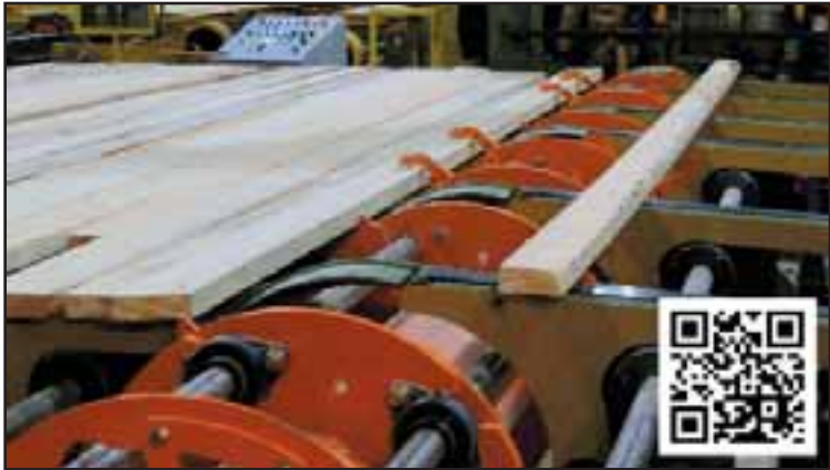
The ElectraTong is USNR's all-electric high-speed lug loader that feeds random length, width, and thickness at 240 lpm.
