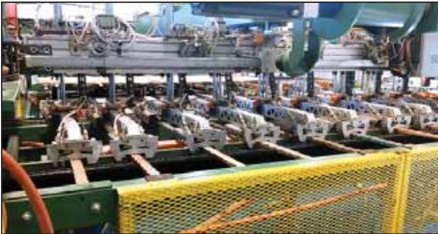
The Accu-Placer grips each stick in two places for precision placement.
