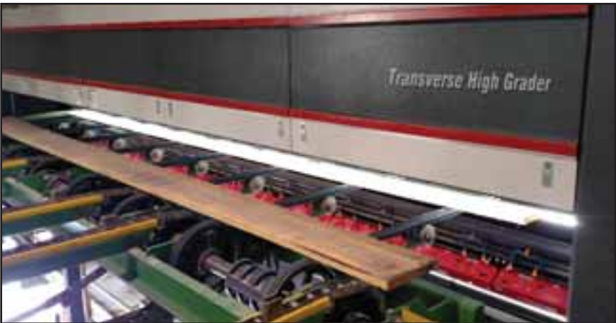
USNR's versatile Transverse High Grader (THG) can be configured for grading dry lumber as well as green flitches and boards. The THG is shown here in a green mill application grading high-value Eucalyptus Grandis.
