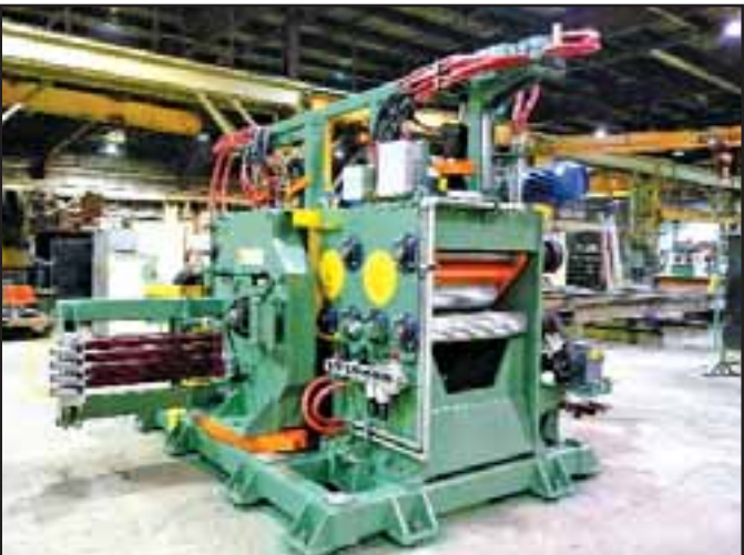
TS Optimized Edgers come in straight, curve sawing, board and gang models.
