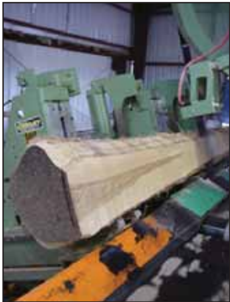
This is a close-up of a Corley tilt carriage at work.
