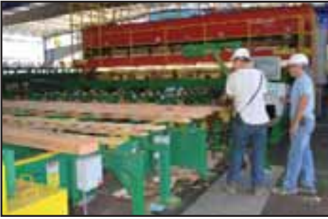
C&D Employees oversee the rotary lug loader that feeds the automatic grade scanner. This scanner is one of the largest in North America.
