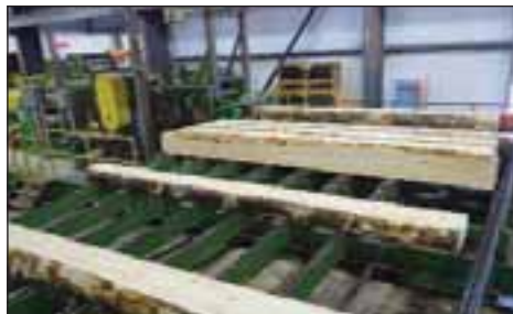
Pictured are White Fir cants lined-up for processing thru Double Arbor Gang-Rip Saw in Empire’s newly rebuilt large log sawmill.
