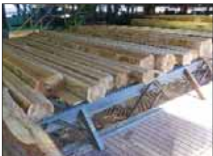
Pictured are cants on the infeed deck to the single arbour 12" gang cluster, along with four shifting saws for boards and up to 10" specialty products.
