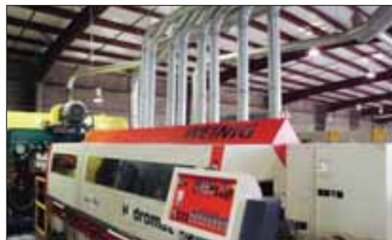
An eight-head Weinig moulder is utilized in the product manufacturing process at Pacific Western.
