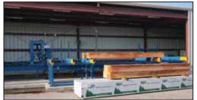
The machine center has the ability to handle timbers as large as 36"x 36" up to 40 feet long at an impressive speed of 1 foot per second.
