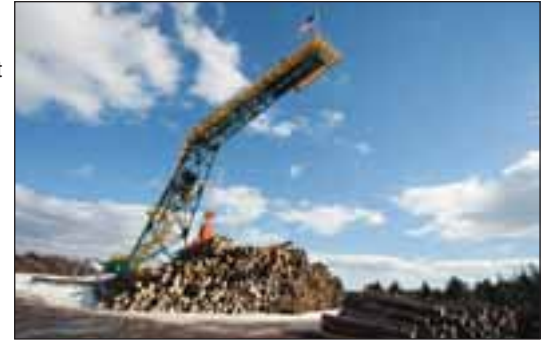
A 25-ton Endurance log crane used in Pleasant River's SPF mill to unload trucks, inventory raw material and load the log merchandising system.
