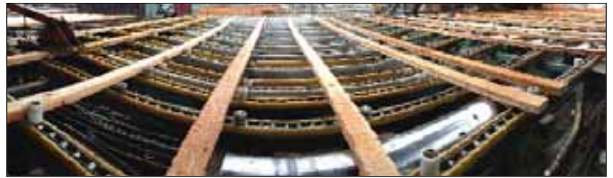
West Bay's production facility has plastic green chain to reduce iron stain.
