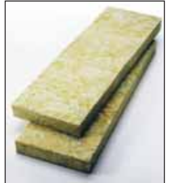
Mineral wool insulation tends to have greater "body" than glass fiber insulation, enabling precise cutting and snug fitting.
